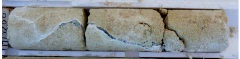
MISTRA and SILACSOL grouts injected in calcarenite (Landfills of Manfredonia, 2010).
