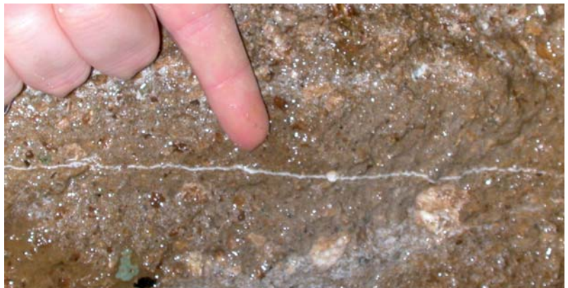
SILACSOL grout injected in tuff (Naples underground, 2007).
