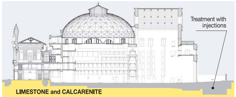
2 - Petruzzelli Theatre, Bari (2004): structural and architectural restoration works - Excavation under the water table with consolidation and waterproofing grouting.
