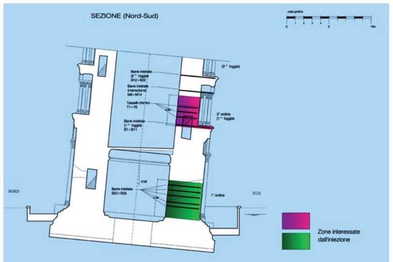
Permanent injection - Tower of Pisa. Consolidation injections of rubble masonry.
